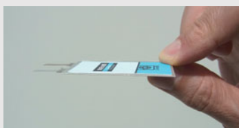
Sheet-type laminated battery (045050 Type)
